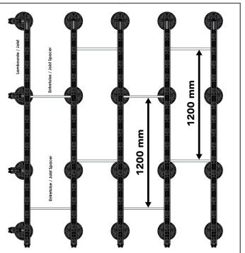
If generic pedestals are used, drill the joist in its groove and fix them together using A2 4x30 (minimum) screws.
