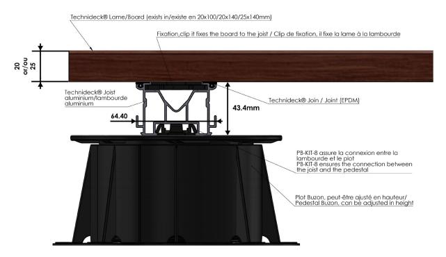
• If **Buzon**<sup>®</sup> pedestals are used, "clip" the PB-KIT8 clip first onto the pedestal in order to be able to fix the *Technideck*<sup>®</sup> aluminum joist with a simple "click". Always secure the first row of pedestals to the joists with a screw. Repeat this operation after each use of the clamping tool (see below: step 8 of the summary of the installation steps).
