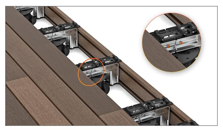
To fix these modules, it is necessary to pre-drill the joist before screwing to prevent breakage. The modules are held using intra-joist connectors and are directly attached using a self-drilling screws at each side.
