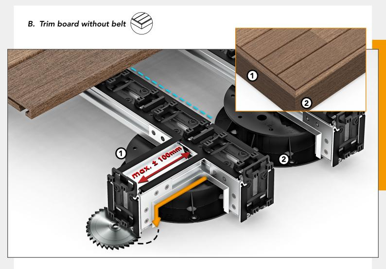
**Cut** the modules as short as possible and fix them perpendicular to the last joist while respecting the axis dimension that was chosen at the start of the installation of the decking.
