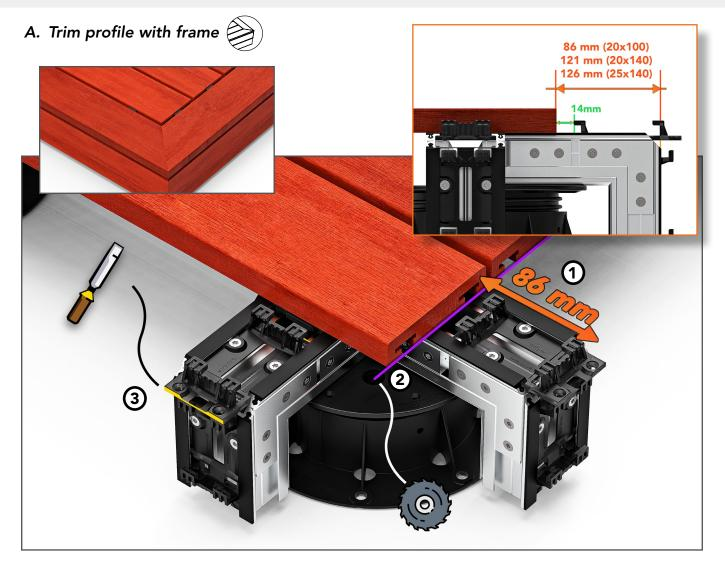
For the trim profile, use the 150mm finishing modules. Cut the joists beforehand in order to arrive just right, making sure to respect the required distances for the belt boards (86mm, 121mm & 126mm: see finishing edge on last page).
