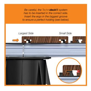
Engage the boards in the fixing clips, the wide side of the board entering the clips, (see opposite drawing). Assemble the planks in the length into each other with the tongue and groove. The 6mm clearance between the boards will be automatically respected by the clip spacer itself. This space has aim to give a correct ventilation of the decking. The next plank must be fully positioned in the fixing clip in order to longitudinally be nested in the previous board's head (see drawing).
