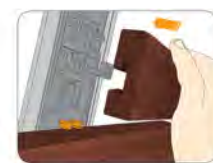
05 Installation of the next wooden board
