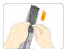
02 Insertion of the <clips> Techniclic® into the bases
